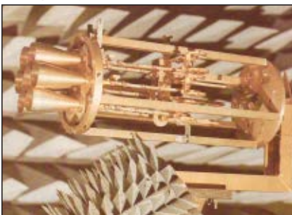
Fig. 1 20 GHz beam-forming network developed by Selenia. ▼
