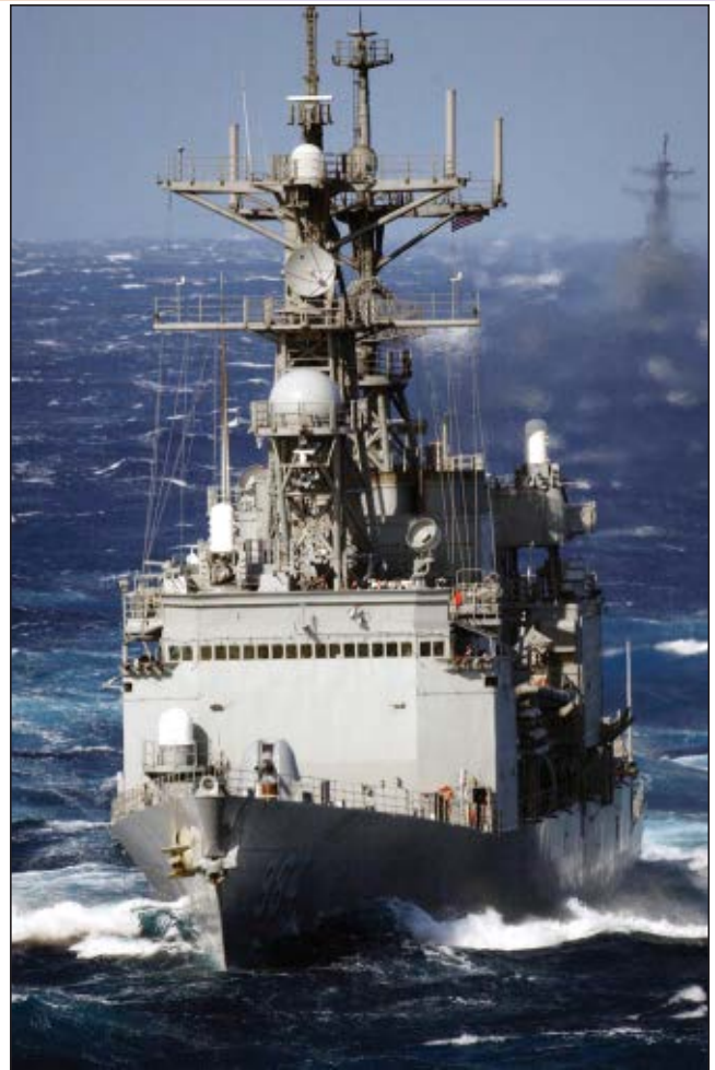
▲ Fig. 2 The ship-based equipment is mounted on the forward and aft masts for diversity.
