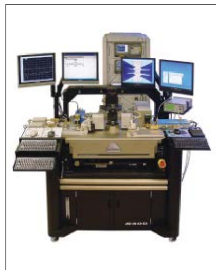
▲ Fig. 3 A WR12 Noise Parameter Measurement System combined with a load-pull system.
